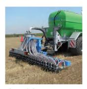
**Slurry injector** Innovative spreading technology
