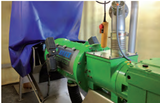
Special press screw separator for BBU
