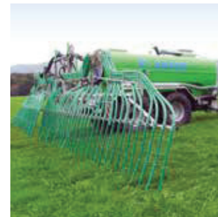
Trailing hose applicator Modular system for all types of tankers
