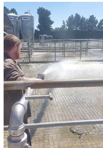
When paired with a 33l/s water pump @ 3Bar the hydrant will achieve a 20-meter radius of cover.
