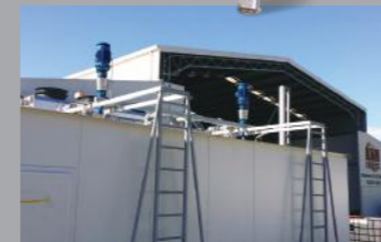
3m long Vertical Stirrers - mixing saltwater ice 24hrs a day
