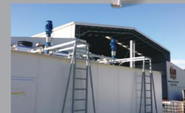
3m long Vertical Stirrers - mixing saltwater ice 24hrs a day
